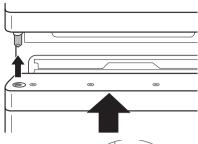
Place the lower door bearing with the bearing pivot in the lower left of the door and fasten.
